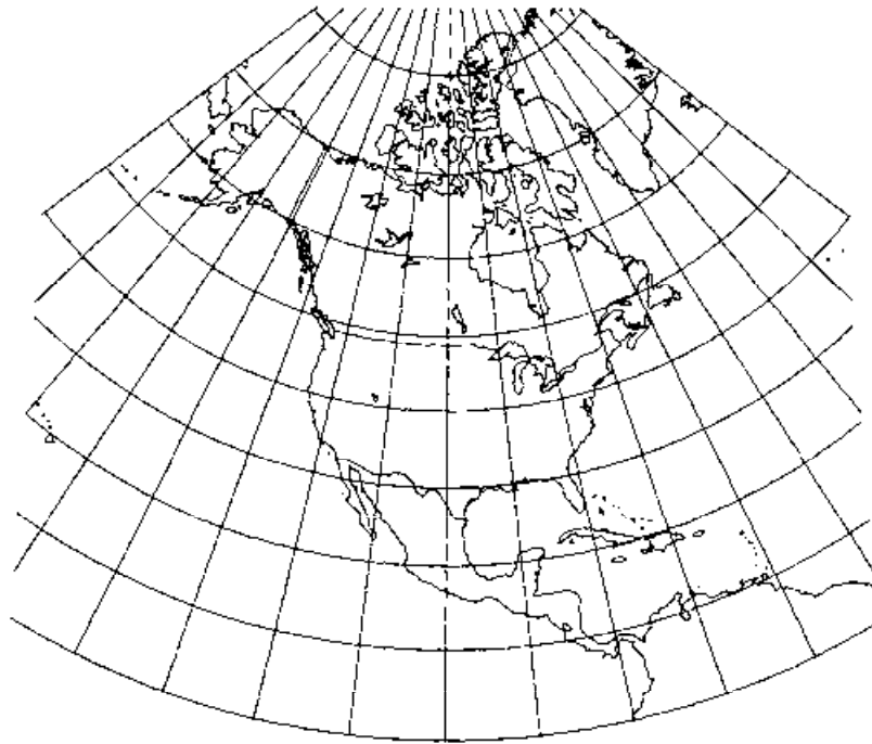
FIGURE 21.—Lambert Conformal Conic projection, with standard parallels 20° and 60° N. North America is illustrated here to show the change in spacing of the parallels. When used for maps of the conterminous United States or individual States, standard parallels are 33° and 45° N.
