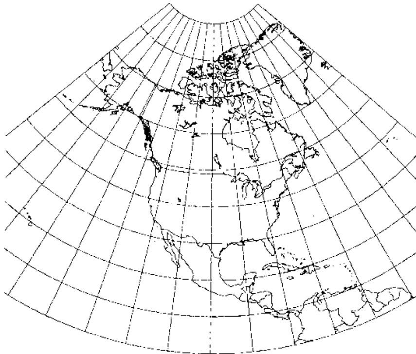
FIGURE 22.—Equidistant Conic projection, with standard parallels 20° and 60° N. All of North America is included to show that parallels remain equidistant. Compare figures 20 and 21.
