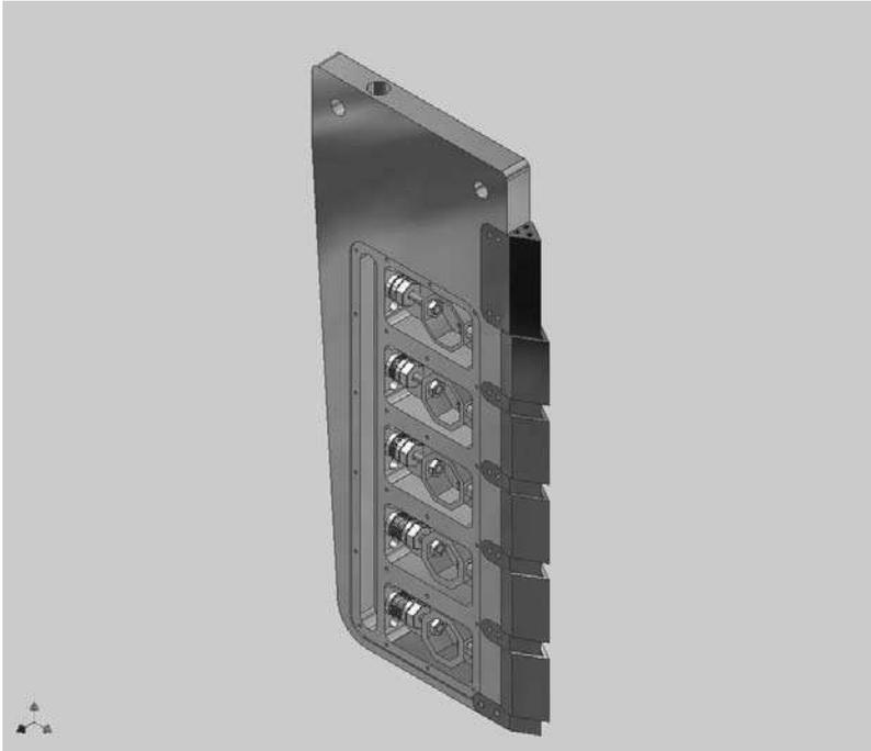
**FIGURE 9.1** CAD drawing of the UCD-SCPS.
